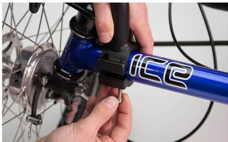
**1** Using a Helping Handle, 1 x bottom plate, 1 x M5 25mm Bolt and a M5 split washer attach the handle on the cross axle, just inside the kingpost.
