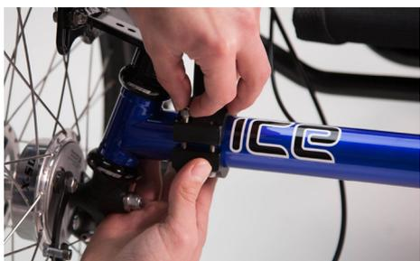
**2** Continue the process for the other 3 bolts, at this point the clamp wants to be tight enough that it doesn't move on its own but loose enough so that you can rotate it with a little pressure.
