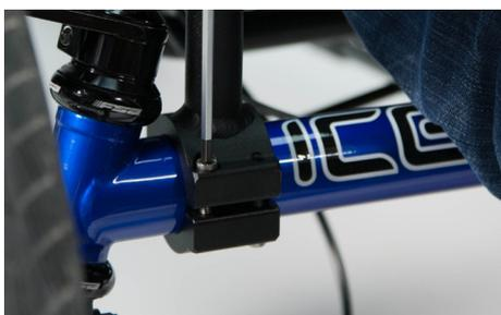
**6** Once you have positioned the Helping Handles continue to tighten all the bolts evenly until you are confident the handles wont slip under your body weight. Overtightening these bolts can do damage to the frame.
