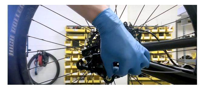
5. Using a Torque Wrench with a 5mm Hex Bit, tighten the Cable stay arm to 4-5 Nm.
