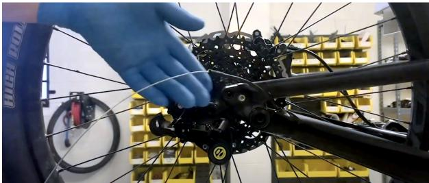
4. Align the Shifter Inner Cable with the channel in the cable stay arm's clamp washer.
