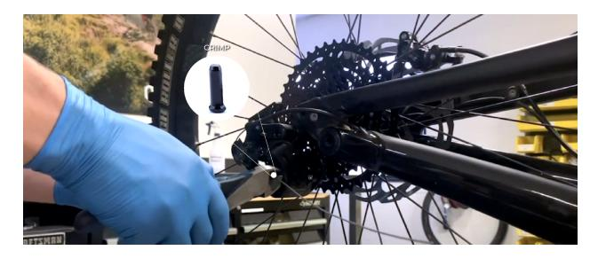
7. Crimp a cable end onto the inner cable to prevent the inner cable from fraying.
