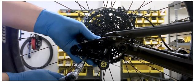
6. Using Cable Cutters, cut the excess cable, leaving 1-2 inches of cable remaining.
