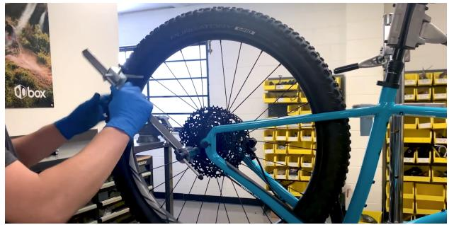
2. Install the rear derailleur to the hanger by using a 5mm Hex Wrench to thread the Derailleur Pivot Bolt onto the hanger. Ensure that the B-Adjust assembly is aligned and set against the derailleur hanger properly.
