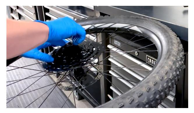
5. Using a cassette lockring installation tool, tighten fully to 40Nm.
