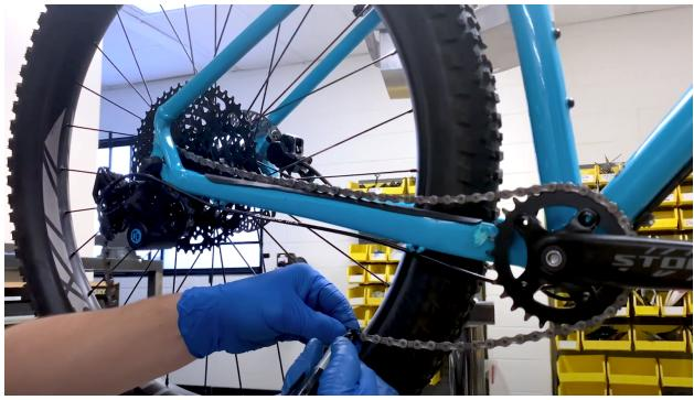
5. Using a -Speed Compatible Chain Breaker, press the marked pin completely out.
