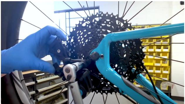
3. Using a Torque Wrench, fully tighten the Derailleur Pivot Bolt to 8-10Nm. Re-check the B-Adjust assembly to ensure there is no gap between the assembly and the derailleur hanger.
