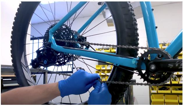
4. With the cage still rotated, identify the two inner links on the chain that meet. Using a marker, mark the link to remove to achieve proper chain length.
