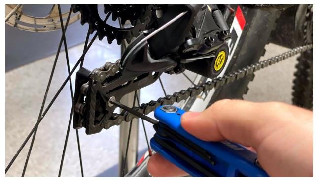
2. Clean the pulleys with mild soap and water or denatured alcohol.
