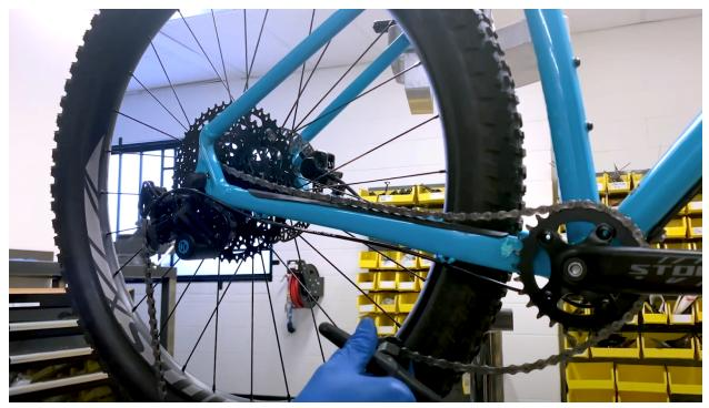
6. Install the outboard connecting link with the "6-8" (or 9S) facing upright and away from the bike.
