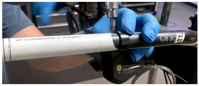
3. Insert the Shifter Inner Cable through the Cable Housing.
