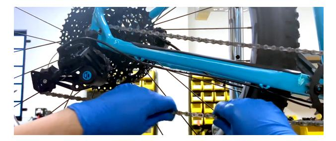
8. Using Master Link Pliers, fully connect the links by pulling the pliers outward.
