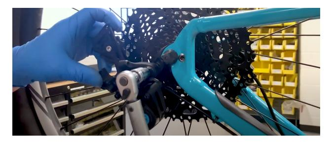
4. Set the High Limit Screw so that the Derailleur's Upper Pulley is inline with the highest cog.
