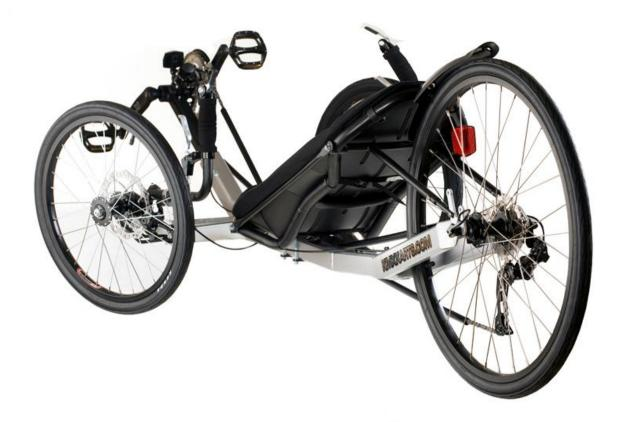
The frame is TIG welded with square chromoly steel tubing and an aluminum boom. Weighing in at 7lbs the Venoms frame is the lightest in the 2011 KMX lineup. The aluminum boom helps reduce the weight and with its design it increases its strength and reduces twisting when pressure is applied. With the low center of gravity, high ground clearance, and frame strength you can take this trike just about anywhere.
