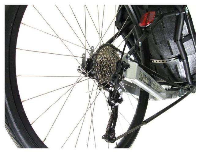
I switched out the stock wheel and cassette with a dual drive, three internal gears and nine external gears. With a ridiculous 81 gears I was able to clime any hill I encountered with ease at just about any low speed. With the same derailleur's I had the same great shifting experience as before, just with more options added in and with the downhill, smooth once again. Not to leave out that I didn't have any shortage of gears on the way down.
